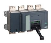
Circuit breaker frame, ComPact NS2000N, 50kA/415VAC, 2000A, fixed, manually operated, without trip unit, 4P
