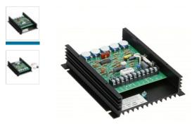
DART CONTROLS DC Speed Control: SCR, Open, 10 A Max Current, 90/180V DC, 50:1, Reversible
