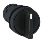
Monolithic selector switch, plastic, black, Ø22, stay put, 2 positions, stay put, 1 NO + 1 NC
