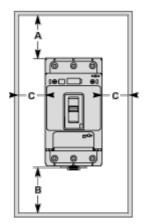
Toggle-type, rotary handle-type: identical clearance values. Safety Clearance (mm)
