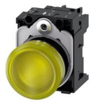
Indicator lights, 22 mm, round, metal, shiny, yellow, lens, smooth, with holder, LED module with integrated LED 230 V AC, screw terminal
