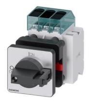
Load disconnector 3LD3, lu 25 A Main switch 3-pole Rated operating capacity at AC-23 A at 400V 9.0kW Front plate mounting Basic switch with Central hole mounting 22.5mm Toggle drive black 48x48 mm with auxiliary switch 1OE + 1S
