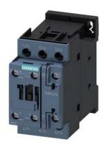
power contactor, AC-3 12 A, 5.5 kW / 400 V 1 NO + 1 NC, 24 V AC, 50 Hz 3-pole, Size S0 screw terminal
