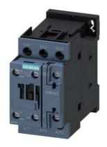
power contactor, AC-3 9 A, 4 kW / 400 V 1 NO + 1 NC, 24 V AC, 50 Hz 3-pole, Size S0 screw terminal
