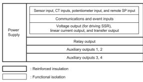
Note: Auxiliary outputs 1 to 2 and 3 to 4 are not insulated.
