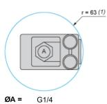
(1) Minimum clearance zone for screwing-on pressure switch at point A
