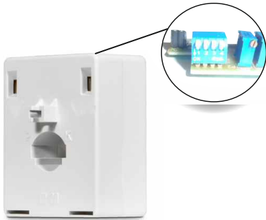
Selection of transformer ratio by switch
