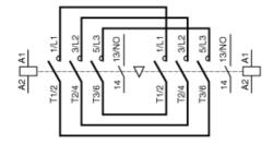
3-Pole Reversing Contactors with Screw Clamp Connections: 3P + N/C
