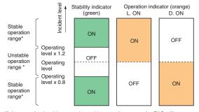
\*If the operating level is set to the stable operation range, the E3G will operate with the highest reliability and without being influenced by temperature change, voltage fluctuation, dust, or setting change. If the operating level cannot be set to the stable operation range, pay close attention to environmental changes while operating the E3G.
