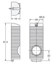
Note: 1. The cover is provided with a rubber bushing and cap to prevent the cable from being pulled out vertically.
